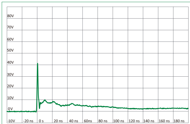
IEC 61000-4-2 +8 kV Contact ESD Clamping Voltage
