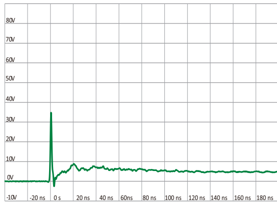
IEC 61000-4-2 +8 kV Contact ESD Clamping Voltage
