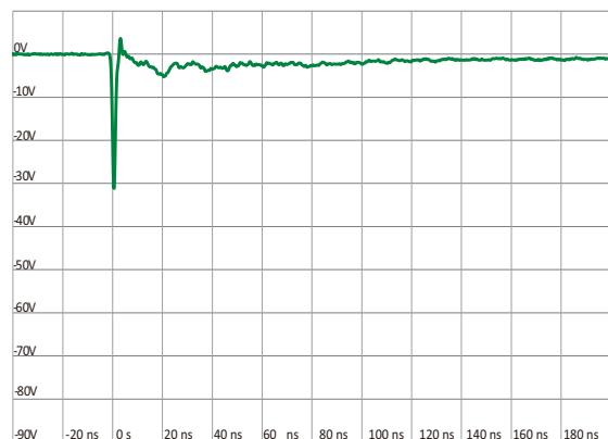
IEC 61000-4-2 -8 kV Contact ESD Clamping Voltage
