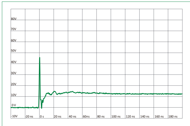
IEC 61000-4-2 +8 kV Contact ESD Clamping Voltage
