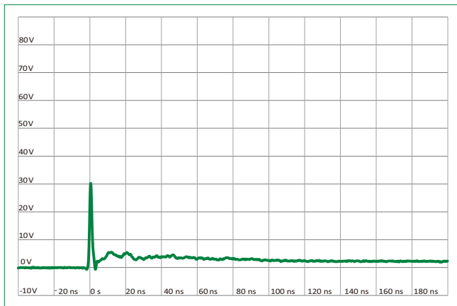
IEC 61000-4-2 +8 kV Contact ESD Clamping Voltage
