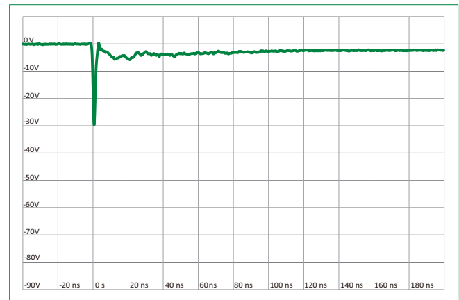
IEC 61000-4-2 -8 kV Contact ESD Clamping Voltage
