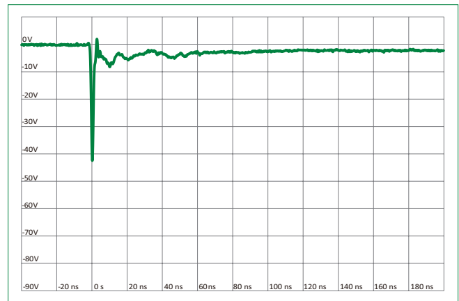
IEC 61000-4-2 -8 kV Contact ESD Clamping Voltage
