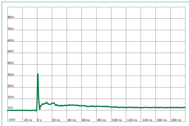
IEC 61000-4-2 +8 kV Contact ESD Clamping Voltage
