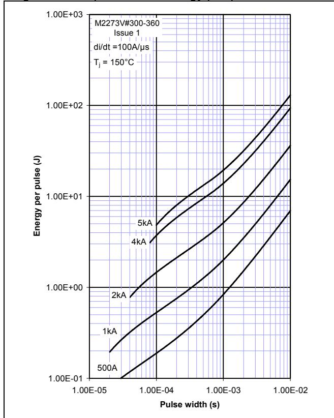
Figure 16 - Square wave energy per pulse
