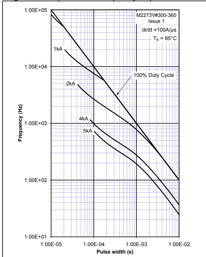
Figure 14 - Square wave frequency vs pulse width
