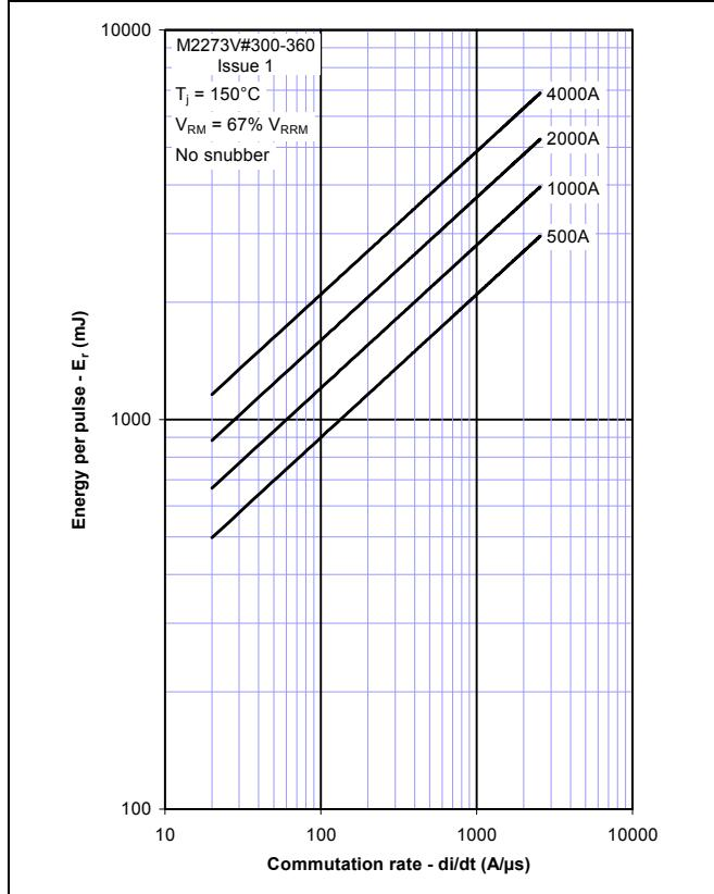
Figure 8 - Sine wave energy per pulse
