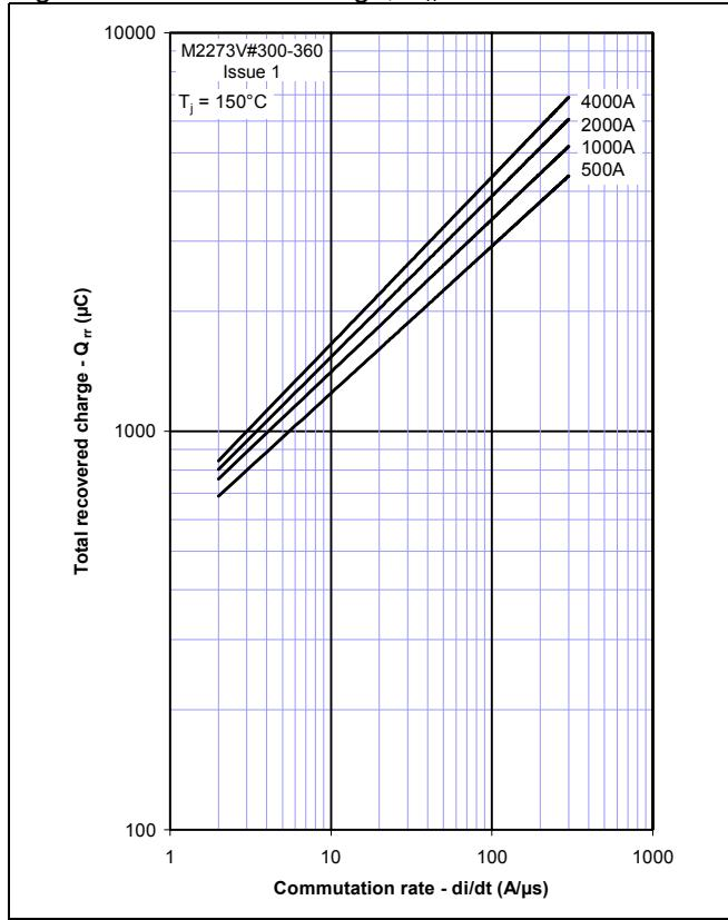
Figure 4 - Recovered charge,  $Q_{ra}$  (50% chord)
