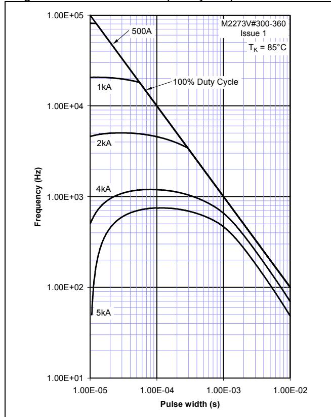
Figure 11 – Square wave frequency vs pulse width
