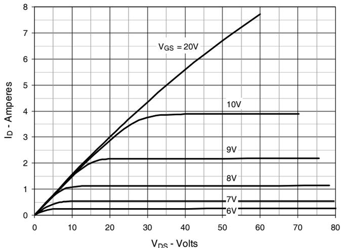
**Fig. 3. Output Characteristics @  $T_J = 125^\circ\text{C}$**
