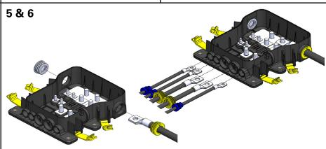
Push the cable assembly through the corresponding input or output slot. Assemble the ring terminal to the stud and secure the cable seal into the housing.
