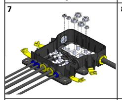
Screw down all the flange nuts onto each stud and to the appropriate torque.
