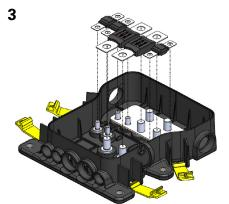
Install the proper MIDI and MEGA Fuses on the top of the busbar and output studs. Ensure the fuse blade is laying flat.
