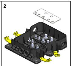
Place the busbar over the input studs in the base
