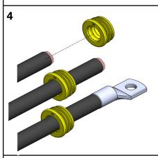
Assemble the properly sized cable seal to the corresponding wire and crimp the appropriately sized ring terminals for each input and output slot. Slide the cable seal a bit past the distance from the stud to the housing slot.
