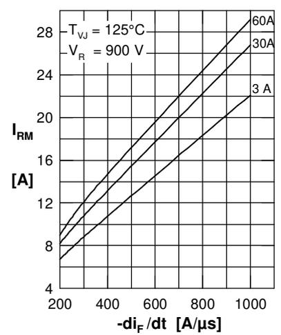
Fig. 3 Typ. reverse recov. current  $I_{RM}$  versus  $-di_F/dt$
