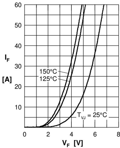
Fig. 1 Typ. Forward current  $I_F$  versus  $V_F$
