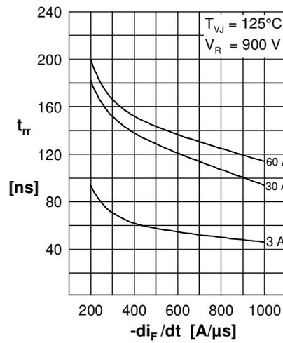
Fig. 5 Typ. reverse recov. time  $t_{rr}$  versus  $-di_F/dt$
