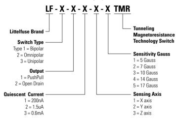
**Example:** LF11115 is Bipolar, Push Pull, 200 nA, X axis, 17 Gauss. **Note:** Every combination is NOT offered. Contact Littelfuse for availability
