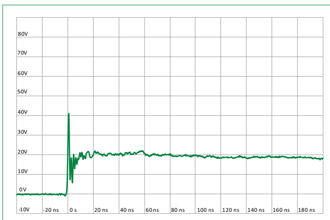
ISO10605 Contact Discharge Plot at +8 kV
