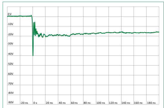
IEC 61000-4-2 -8 kV Contact ESD Clamping Voltage
