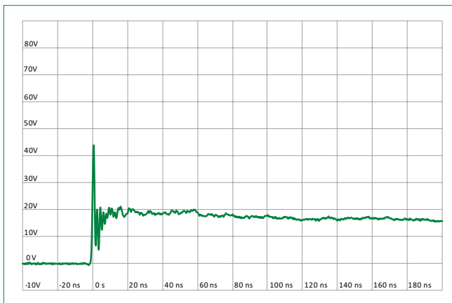
IEC 61000-4-2 +8 kV Contact ESD Clamping Voltage
