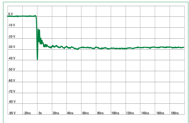
ISO10605 Contact Discharge Plot at -8 kV
