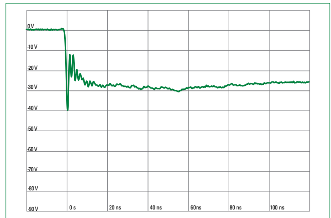
IEC 61000-4-2 -8 kV Contact ESD Clamping Voltage
