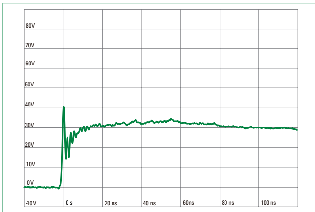
IEC 61000-4-2 +8 kV Contact ESD Clamping Voltage
