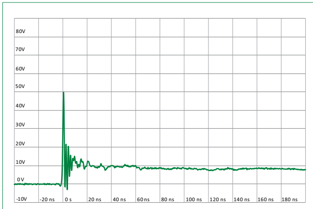
IEC 61000-4-2 +8 kV Contact ESD Clamping Voltage
