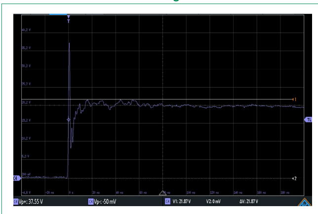
SC1122 IEC 61000 -4-2 +8 kV Contact ESD Clamping Voltage
