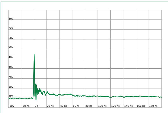
IEC 61000-4-2 +8 kV Contact ESD Clamping Voltage
