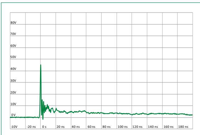
ISO10605 Contact Discharge Plot at +8KV
