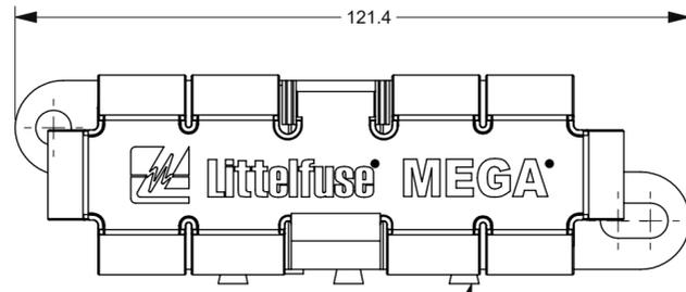
DOVETAIL FEATURES USED TO INTERLOCK MULTIPLE HOLDERS
