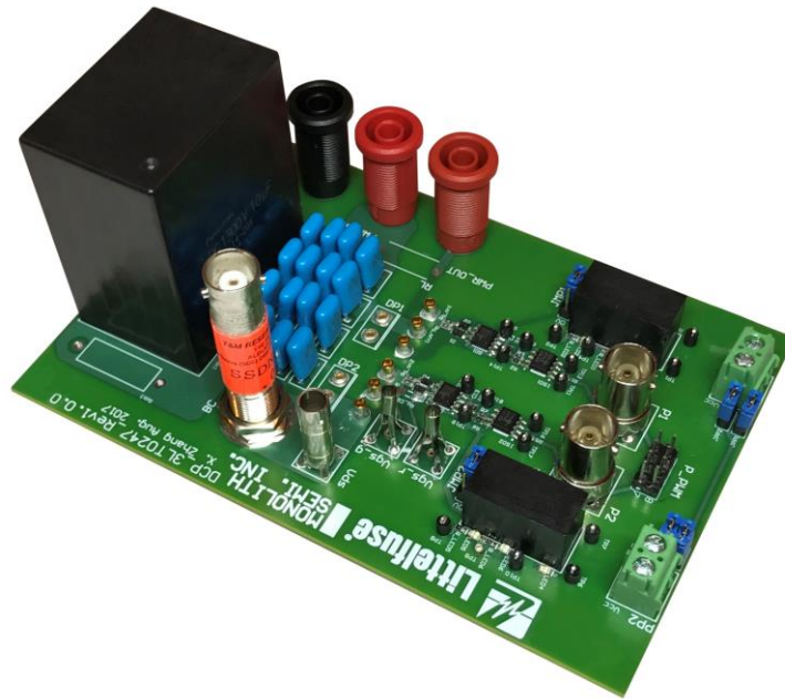
Figure 3. Dynamic Characterization Platform Assembly
