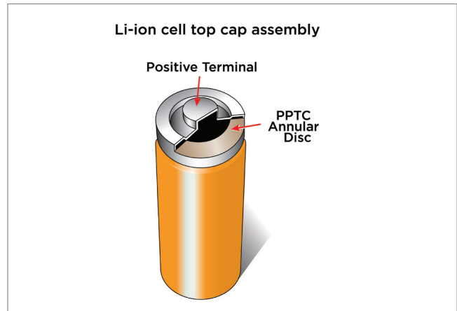
Figure 8. A PolySwitch disc device's placement on an 18650 battery cell.
