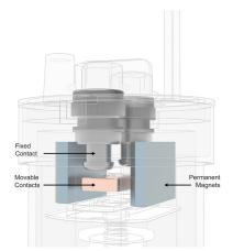
Double-opening contacts effectively double the opening distance based on the same motion of the moving contact bridge.
