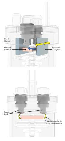
Magnetic blowouts effectively lengthen the opening distance by forcing the path of the arc to the outer edge of the contact chamber along magnetic field lines created by permanent magnets in the contact area. The magnetic field lines interact with the arc by charge, so the arrangement of the magnets determines how effective the magnets are in extending the path of the arc.
