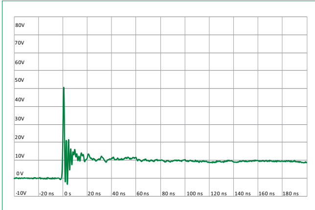
ISO10605 Contact Discharge Plot at +8 kV
