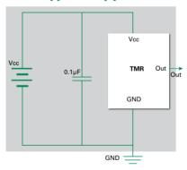
Note: It is strongly recommended that an external bypass capacitor be connected in-close-proximity to the device between the supply and ground pins to reduce noise. The recommended value for the external bypass capacitor is  $0.1\mu F$ .
