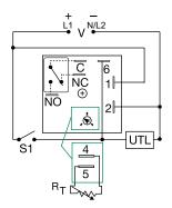
V = Voltage S1 = Initiate Switch C = Common, Transfer Contact NO = Normally Open NC = Normally Closed
