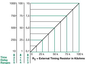
This chart applies to externally adjustable part numbers. The time delay is adjustable over the time delay range selected by varying the resistance across the  $R_T$  terminals; as the resistance increases the tie
