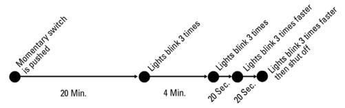
Any time the momentary switch is pressed, the sequence is restarted.
