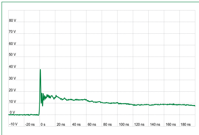
IEC 61000-4-2 +8 kV Contact ESD Clamping Voltage
