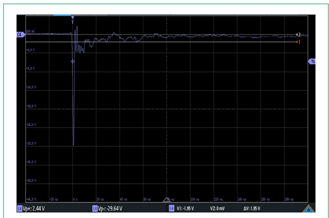
SC1122 IEC 61000 -4-2 -8 kV Contact ESD Clamping Voltage
