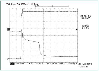
Channel 1: current through LEDs (346 mA) and PLED device once it is fully turned on 2.5  $\mu$ sec later Channel 2: voltage across PLED device (21.3 V before PLED crowbars with 2 V drop)
