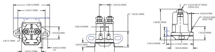
Shown: Insulated solenoid with 5/16" studs and two coil blade terminals.
