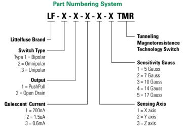
**Example:** LF11115 is Bipolar, Push Pull, 200 nA, X axis, 17 Gauss. **Note:** Every combination is NOT offered. Contact Littelfuse for availability.
