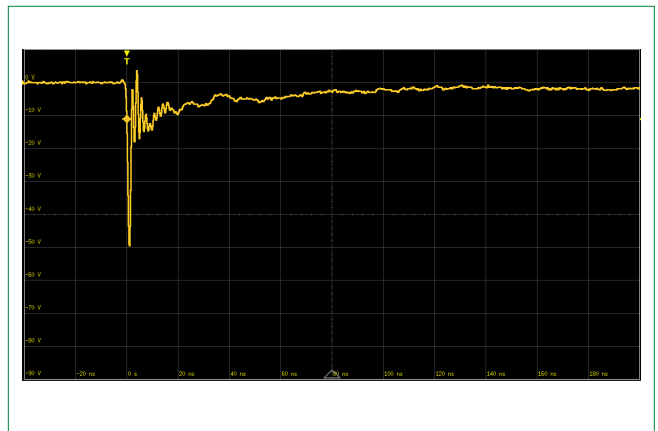
IEC 61000-4-2 -8 kV Contact ESD Clamping Voltage
