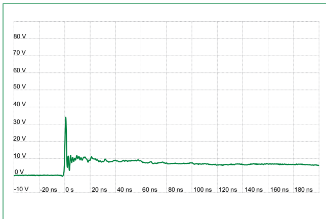
IEC 61000-4-2 +8 kV Contact ESD Clamping Voltage
