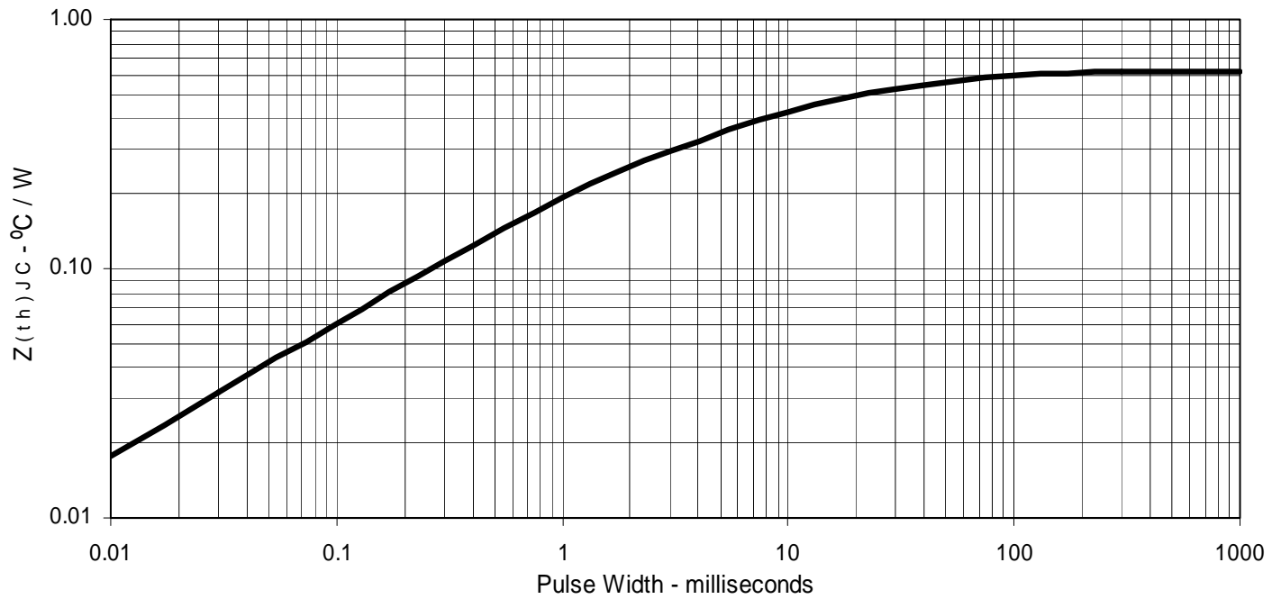
Fig. 13. Maximum Transient Thermal Impedance
