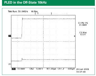
Channel 1: current through LEDs (318 mA) Channel 2: voltage across PLED device (4.5 V)
