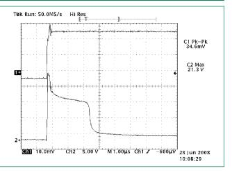
Channel 1: current through LEDs (346 mA) and PLED device once it is fully turned on 2.5  $\mu sc$  later Channel 2: voltage across PLED device (21.3 V before PLED crowbars with 2 V drop)
