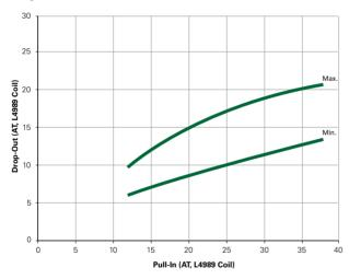
**Note:** Chart represents the range of Drop-Out, min to max, for a given Pull-In value of the MDCG-4 prior to modification into the MDSM-4.
