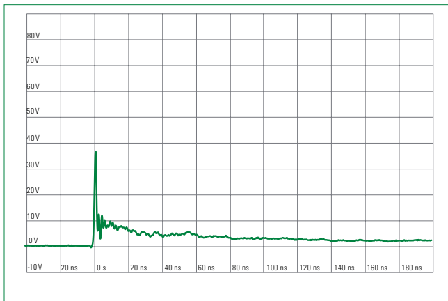
IEC 61000-4-2 +8 kV Contact ESD Clamping Voltage
