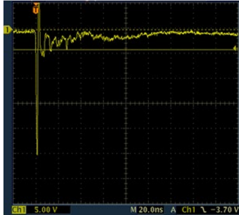
SP1124 IEC 61000 -4-2 -8 kV Contact ESD Clamping Voltage
