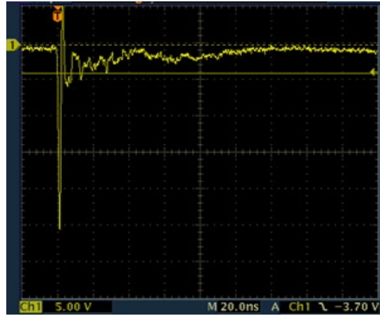
SP1112 IEC 61000 -4-2 -8 kV Contact ESD Clamping Voltage
