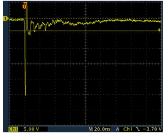
SP1112 IEC 61000 -4-2 -8 kV Contact ESD Clamping Voltage
