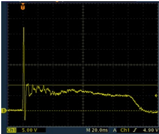
SP1112 IEC 61000 -4-2 +8 kV Contact ESD Clamping Voltage
