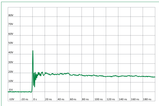
IEC 61000-4-2 +8 kV Contact ESD Clamping Voltage
