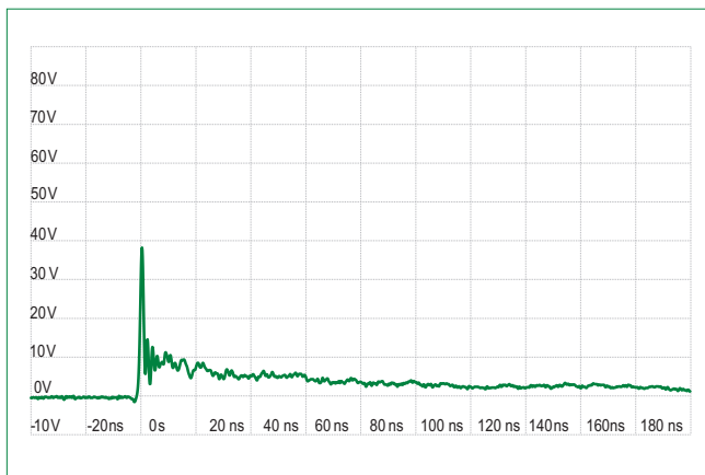
IEC 61000-4-2 +8 kV Contact ESD Clamping Voltage
