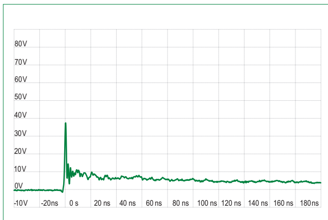
ISO10605 Contact Discharge Plot at +8 kV
