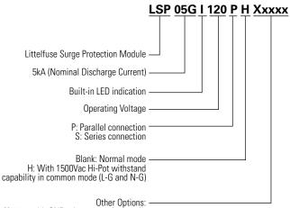
X333: with GND wire connection, available for 240Vac and 277Vac rating with CE Marking for Class I earthed luminaire installation Wire Color: Line: Brown, Neutral: Blue, Ground/PE: Green with yellow stripe
