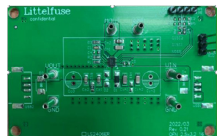
Figure 6. LS2406ERQ23 EV. Board 28V, 6A with Reverse Current Blocking
