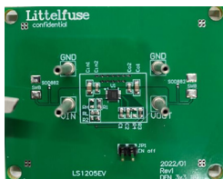
Figure 5. LS1205EVD33 EV. Board 12V/5V/3.3V with Programmable OCP / OVP
