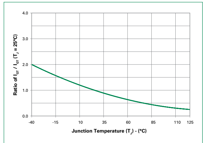
Figure 2: Normalized DC Gate Trigger Current vs. Junction Temperature (Standard SCR)
