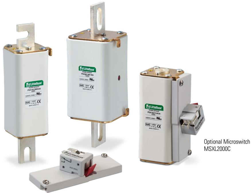
The PSX series high-speed fuses deliver extremely fast-acting performance up to 1500 V dc. Available in flush-end, DIN-mount, and bolted-blade styles, they are the smallest NH XL package size on the market and range from 80 A to 1400 A. The PSX series is extremely fast-acting with 250 kA dc interrupting ratings. Visual blown fuse indication is standard on all fuses and an optional micro-switch is available for external indication.
