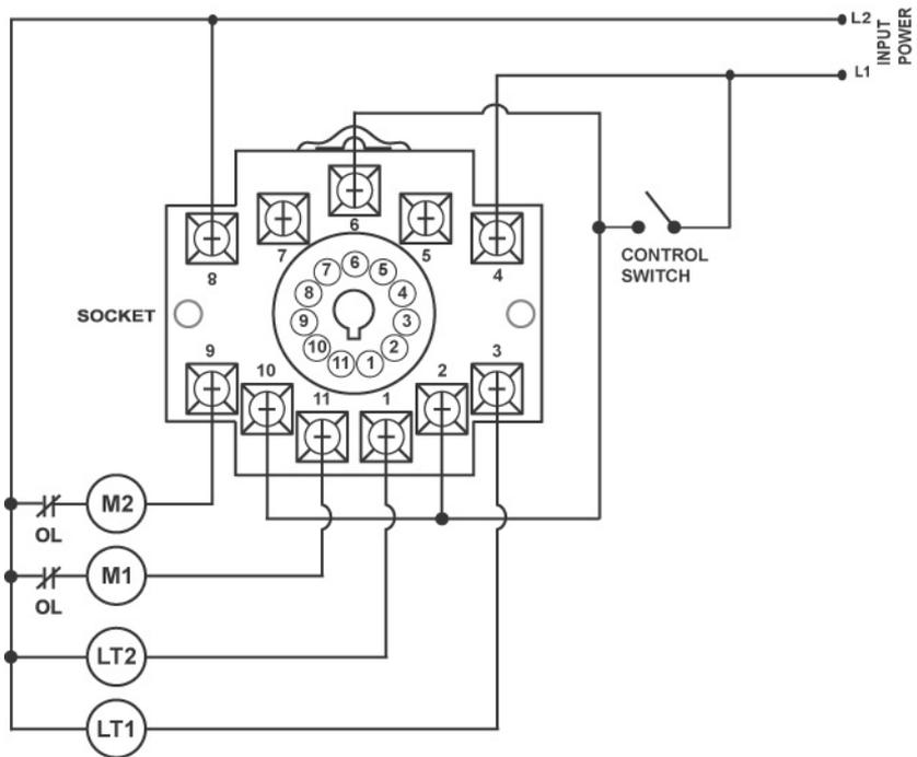
Figure 2: Typical Pump Control Wiring Diagram
