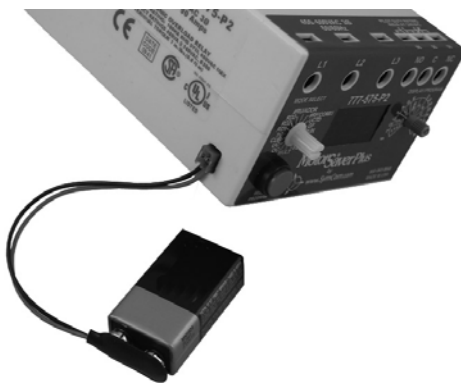
Figure 3: Proper Position of the Battery Cable
