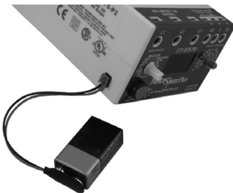
Figure 4: Proper Position of the Battery Cable
