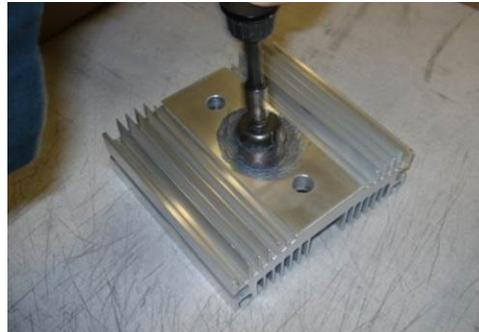
Note that the rotary wire brush must be replaced when the bristles are too short.
