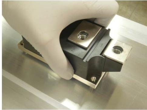
Torque the screws to the correct torque wrench setting as detailed in the datasheet.
