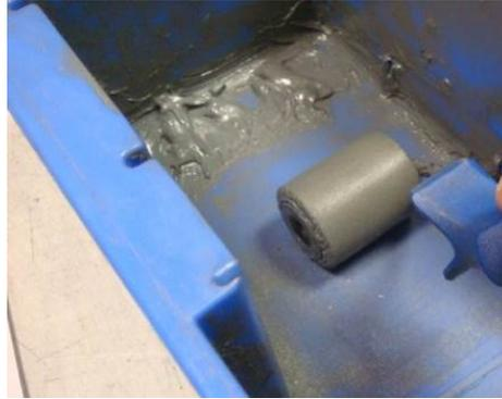
Apply the grease to the heatsink close to the spiro pin as shown.
