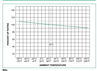
Rerating depicted in this curve is in addition to the standard derating of 25% for continuous operation.
