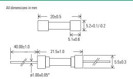
\*Rating of 20A has 1.20±0.05 diameter lead
