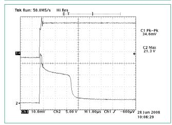
Channel 1: current through LEDs (346 mA) and PLED component once it is fully turned on 2.5 µsec later Channel 2: voltage across PLED component (21.3 V before PLED crowbars with 2 V drop)
