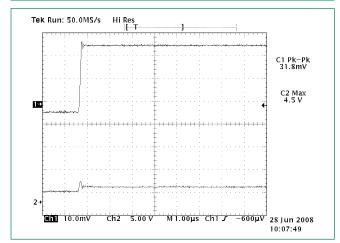
Channel 1: current through LEDs (318 mA)
