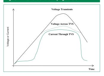
Figure 2 - Peak Pulse Power Rating
